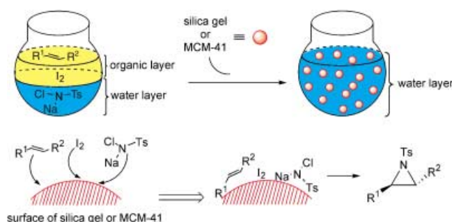
Figure 1. Proposed path for the formation of aziridines in a water–silica system.
